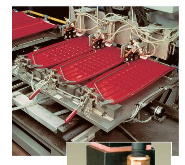
Automated gasketing is beneficial to virtually any gasketing application from automotive taillights to electrical enclosures to window backbedding and appliance seals. Manufacturing processes from semi-automated, single-item production to fully-automated, continuous production lines will benefit from automating gasket placement.
