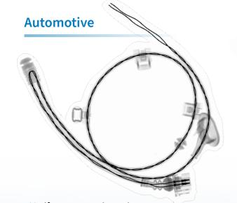
Verify connector integrity and sufficient wire pair twisting in cable assemblies.
