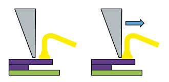
Figure 4. Step back of the shear tool followed by bond shear
