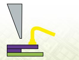
Figure 1. Alignment of shear tool with ball bond
