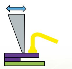
Figure 3. Shear tool being slowly raised until oscillating force is reduced to zero
