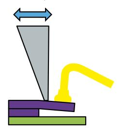
Figure 2. Shear tool lands and oscillates producing a measurable force on the transducer
