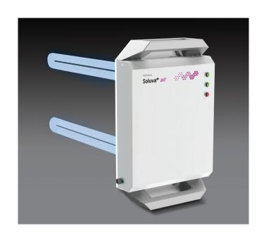
Soluva® Air D modules are available in four different lengths for installation in all common return air ducts. The modular system design enables the installation of several modules next to each other to achieve the required radiation dose based on the dimensions of the ducts and the air velocities.
