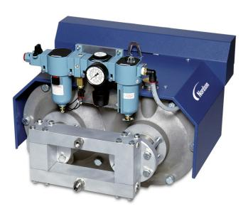
The Nordson model DR pump is an air-driven pump for use in the application of waterborne container coating materials and can be used in both heated and unheated delivery systems. Developed specifically for the container industry, the demand-type, dual-piston DR pump maintains constant fluid pressure throughout the pumping cycle to achieve the superior overall performance required in high-speed can coating applications.
