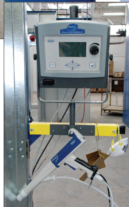
(Above) VentCore bake oven and controls. (Right) High Density Powder Low Volume Air (HDLV) spray gun and control system.
