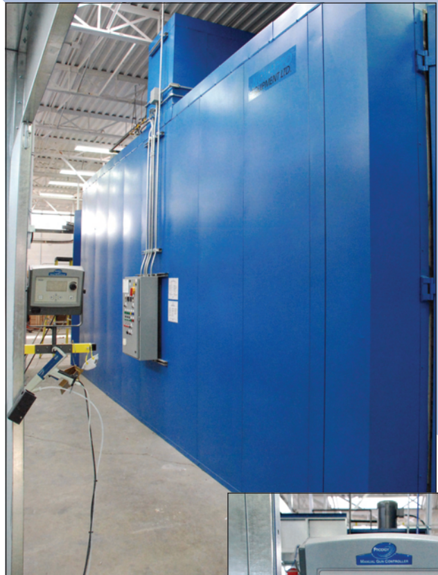
(Above) VentCore bake oven and controls. (Right) High Density Powder Low Volume Air (HDLV) spray gun and control system.
