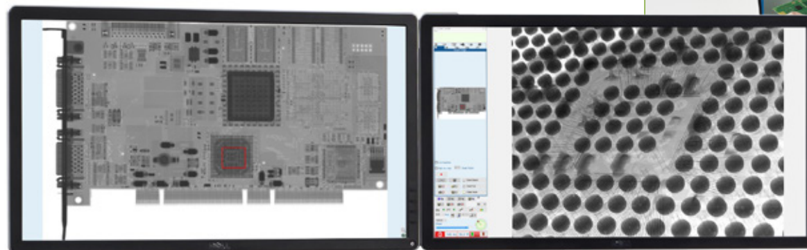
Sample navigation and fault location map. Quickly magnify any component by drawing a rectangle around it.
