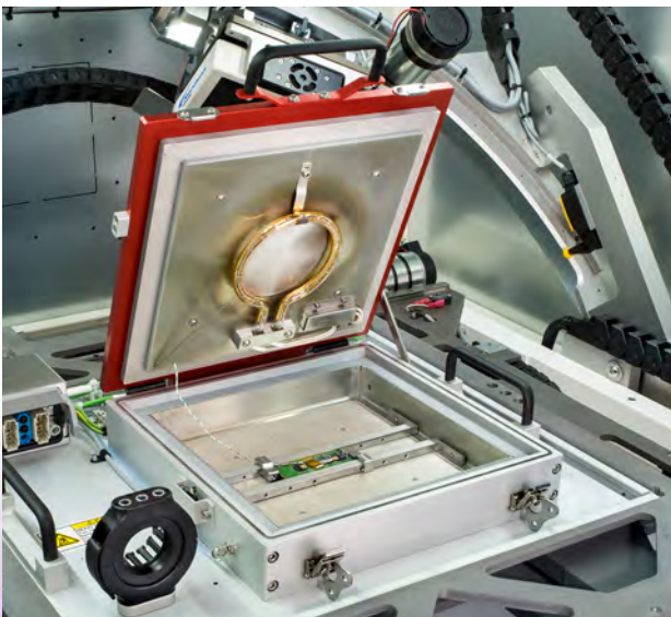
Figure 1 : Heated Stage Reflow Simulator inside Quadra X-ray Inspection System.
