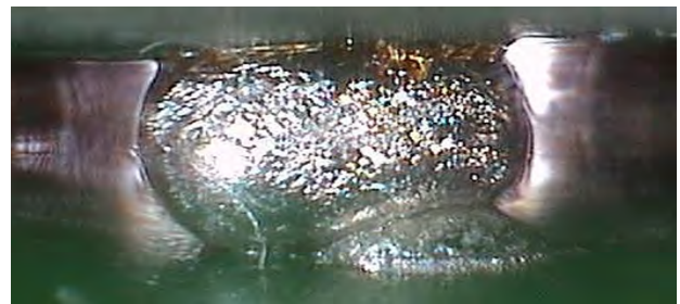
Figure 2: Optical image of a HIP defect.
