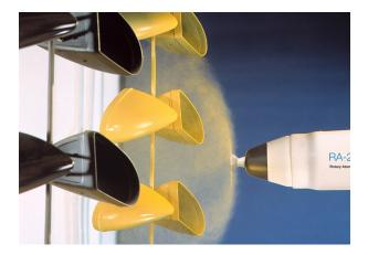
With the RA-20, spray patterns can be adjusted from eight to 42 inches wide, depending on the coating material used. This allows for application of a precise amount of paint with minimal overspray with less paint waste and lower clean-up costs.
