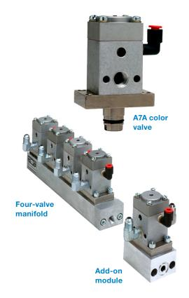
Nordson Model A7A color-change valves deliver fast and reliable color-change performance for improved productivity and maximum operating efficiency. They respond to pneumatic signals and feature a carbide ball and seat for positive shut-off and long service life when used in abrasive coating applications. The A7A valves can also be used with custom-designed manifolds.
