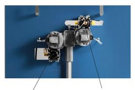
Solvent valves on base and catalyst manifolds provide a complete flush Adjustable stroke limit allows user to set catalyst injection rate
