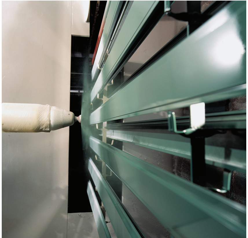
Nordson Rotary atomizers accommodate a multitude of part profiles, handle frequent color changes, match colors consistently and continuously, provide a quality finish and minimize paint waste and touchup.
