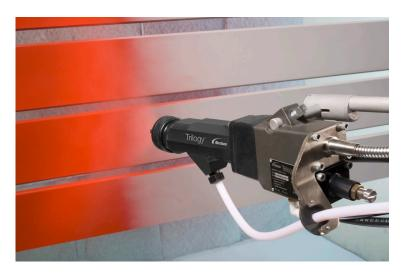
the velocity to penetrate recesses and corners on the extrusions for consistent primer coverage.
