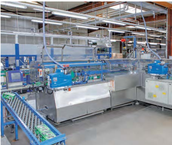
The packaging machine – shown with the hood open for better visualisation – with a full view of the two new ProBlue Liberty hotmelt application systems mounted at chest height.
