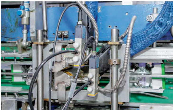
The end gluing of showboxes is performed on both sides using two multi-module MiniBlue II dispensing guns.
