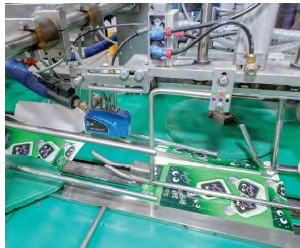
The longitudinal edge is glued by a fully insulated pneumatic MiniBlue II Slim Line applicator.
