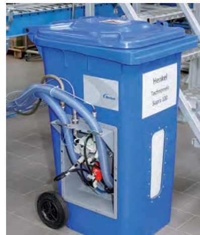
With the multifeeder option, hot melt is supplied to both ProBlue Liberty systems simultaneously from the large-volume 240-litre storage container.
