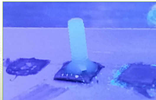
Figure 1 Nylon stud being bonded to a silicon die curing under a UV lamp
