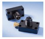
Nordson EFD's two-component manifolds separately port the resin and hardener into the mixing nozzle. Cleanup simply involves wiping the manifold face after the nozzle has been removed.
