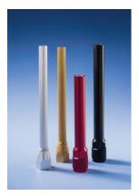
For medium- and high-pressure systems where pressure inside the mixer is greater than 10 bar (150 psi), we recommend that a metal jacket be used over the mixing nozzle. Nordson EFD offers a range of low-cost, one-piece jackets. Select Robotic version where repeat positioning is required.
