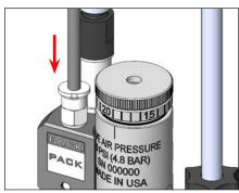
Step 3. Connect air input hose 4.8–6.2 bar (70–90 psi) into 4 mm push-in fitting.
