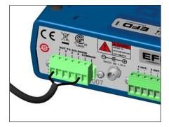
Step 4. Interconnect the BackPack to the ValveMate™ 8000 Controller using the cable supplied.
