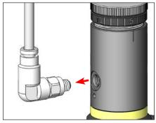
Step 1. Remove actuation air fitting and hose from air cylinder body.
