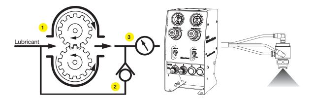
**IMPORTANT NOTICE:** Caution should be used when selecting a lubricant to use with the MC600M system. Fluids with a flash point lower than 38° C (100° F) are not recommended, as they could present a fire hazard. Examples of products with low flash points are kerosene, acetone, general mineral spirits, naphtha, and other solvents. Please check the product SDS carefully before using the intended product in this system.
