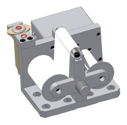
PICO® Jet Valve Cleaning station for mechanically cleaning the exterior of dirty nozzle plates.
