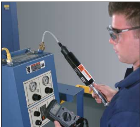
Flexible cable attachment measures voltage inside high-voltage power supply for powder (left) and liquid (right) coating application systems.
