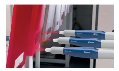
Encore HD guns are perfectly suited for use with the ColorMax® fast-color-change powder coating and recovery booth systems. Providing reclaim-to-reclaim color change in generally 5 to 10 minutes, the ColorMax system also ensures optimum application area air flow and control for maximum coating performance and efficiency in today's lean manufacturing operations.
