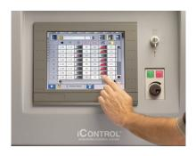
The iControl system can accept input from part identification sensors for gun triggering and in/out positioning, and can accommodate up to 255 presets. These presets can be tailored to each color and each part for substantial powder material savings
