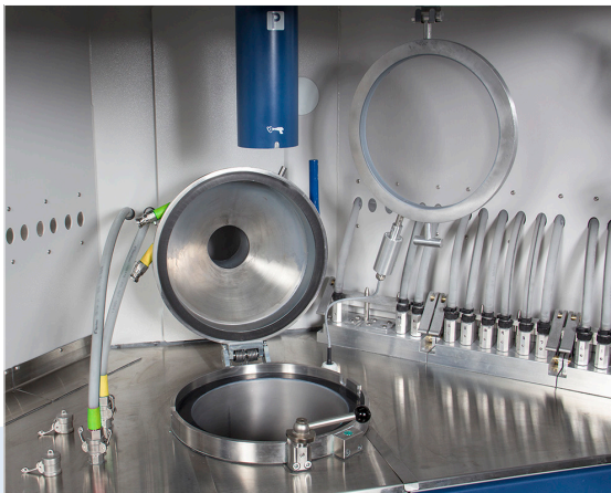
Cylindrical hopper design eliminates difficult to clean corners
