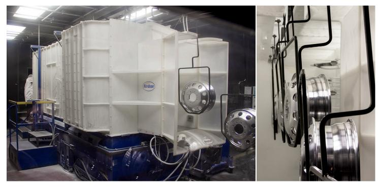
The Nordson Horizon 400 downdraft booth ensures optimized air flow and application efficiency
