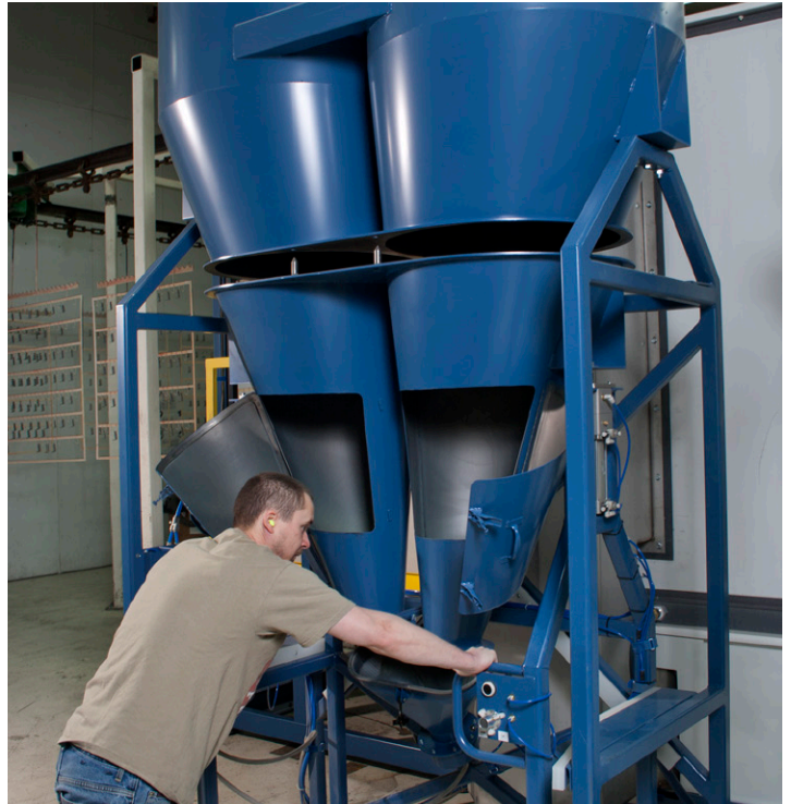
Aesthetic Finishers' newest powder coating system has a dual cyclone design that maximizes cleaning efficiency. To accommodate more challenging powders, the cyclone's lower section can be unclamped and rolled out, allowing the cyclone's entire interior surface to be easily wiped clean from top to bottom.
