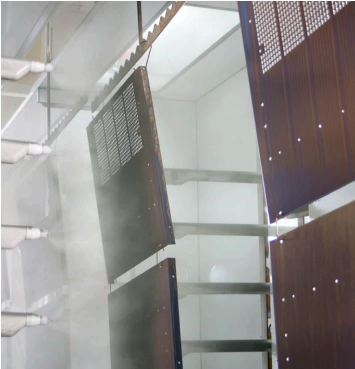
As one of Ohio's largest powder and ceramic coating facilities, Aesthetic Finishers caters to industries that require the highest quality finishes. Here, appliance parts are being sprayed, just one job of the hundreds of parts that are coated each week in more than 50 different colors, at the shop's 80,000 sq.-ft. facility..
