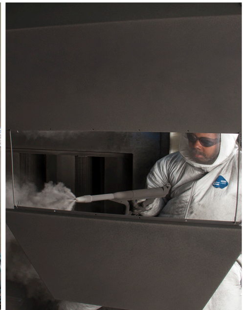
An operator manually reinforces parts in an Excel® 2000 series booth in the "Line 2" facility.
