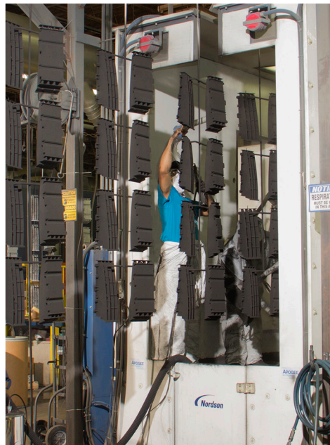
Operators manually touch-up parts in the Nordson Colormax system in the "Line 1" facility.
