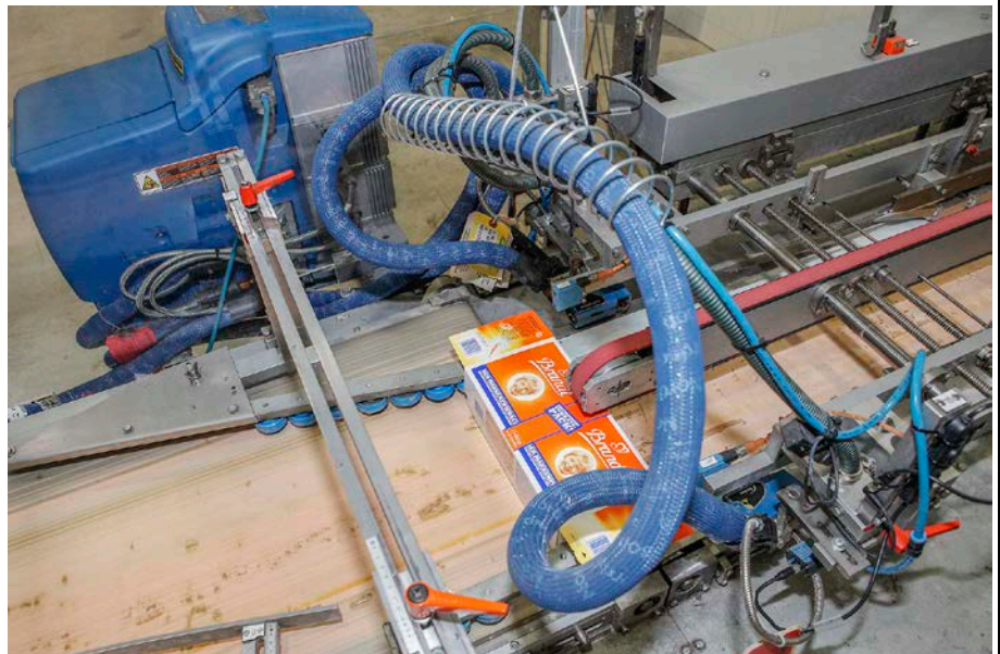
Detail view of front flap gluing (photo: Kimberly Wittlieb)
