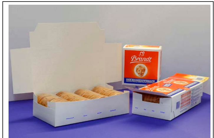
Using the EcoBead application controller, the previously continuous hot melt beads for front and side flap gluing were divided into four sequences each, saving considerable material. The transparent strips of hot melt are shown blue in the picture for better visualization (photo: Kimberly Wittlieb)
