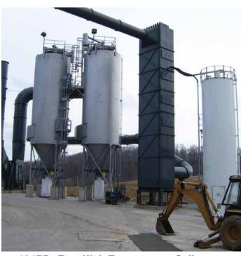
484RF - Two High Temperature Collectors on Secondary Aluminum Processing
