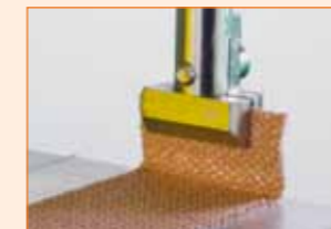
Wider tweezers provide better grip on wide samples
