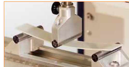
Assessing the flexural modulus and strength of composites using a three point bend test
