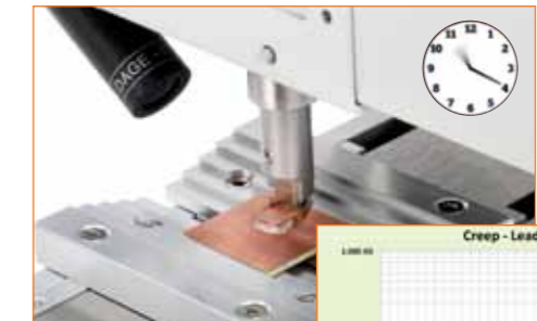
Slow deformation of solder at room temperature
