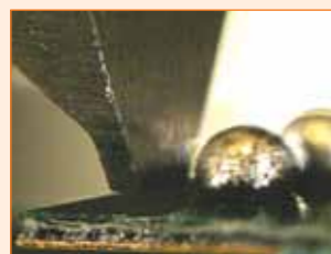
Accurate shear heights are guaranteed by light touch down control
