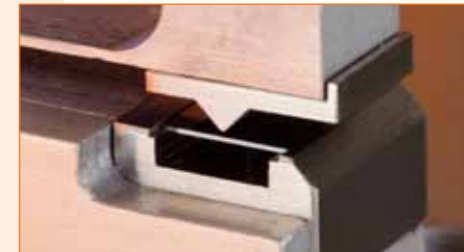
Custom tooling for micro bend eases sample placement and produces repeatable data
