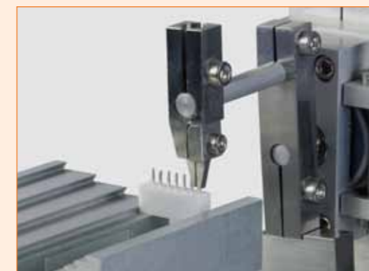
Subjecting the legs of a connector to bend and twist
