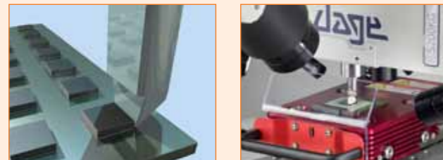
Shear tests can be performed on samples from microns to centimetres in size
