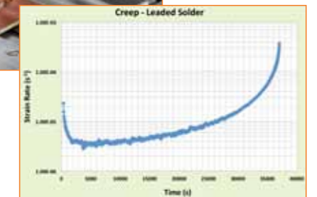
Slow deformation of solder at room temperature
