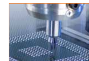
Sample firmly gripped for high speed pull test
