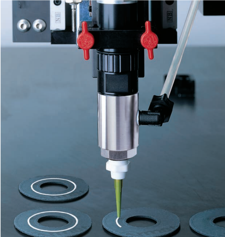
725DA dispensing even bead of water-based adhesive.
