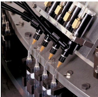
741V valves dispense UV-cure on a medical production turntable.
