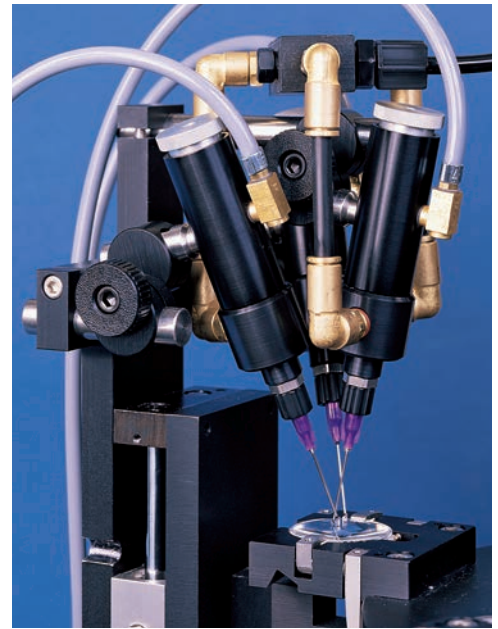
741V valves dispense dots of UV-cure adhesive on a bar code scanner lens.
