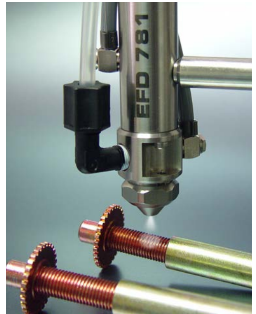
781S sprays lubricant on automotive brake adjusters.
