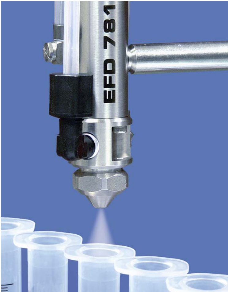
781S spray valve uses low volume low pressure (LVLP) technology to apply a fine coating of silicone oil inside medical syringes.
