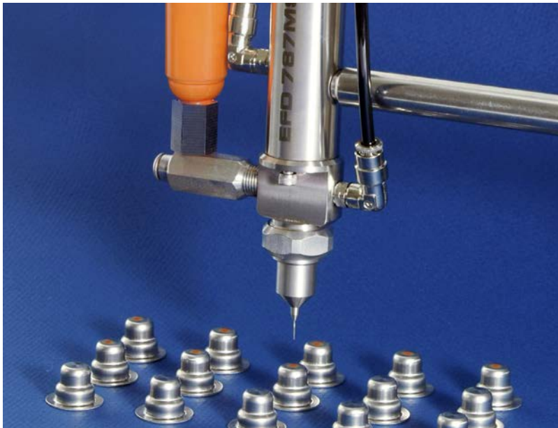
Apply a precise, uniform spray pattern more than 30% smaller than standard spray valves.
