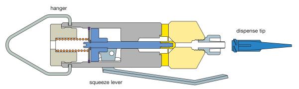
**Note:** The fluid input fitting is located 90° from the squeeze lever.
