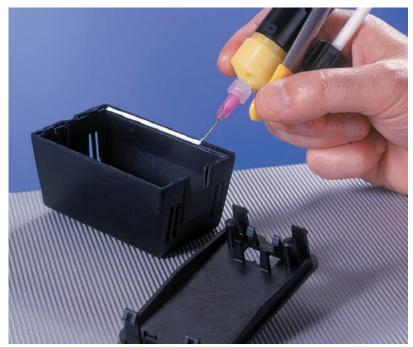
Handheld dispense valves are a good choice for manual assembly applications where a timed shot is not required and a relatively large amount of fluid is being applied.
