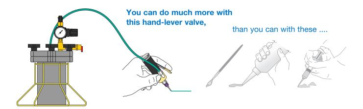
Set the fluid reservoir pressure at the exact flow you need. Then position the dispense valve and get precise beads ... exact, neat, fast and without mess, waste or rework. EFD reliable dispense hand-lever valves take the fuss out of assembly fluid dispensing.
