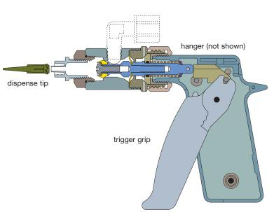
Designed for heavy duty operation, the 725-HL provides relatively high flow application of mediumto high- viscosity nonreactive fluids without fuss, maintenance or downtime. Accepts dispense tips, and larger metal and plastic nozzles.
