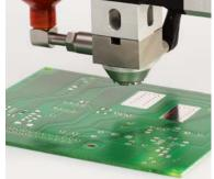
Non-contact micro-dispensing of beads and fills onto hard-to-access or delicate surfaces is easy and repeatable.
