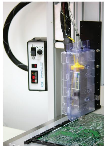
Maintains temperature-sensitive dispensing processes within  $\pm 0.1^{\circ}$ C of a desired set point, across a 10° to 40°C range.
