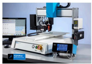
NX protocol via Ethernet allows programming from a personal computer or PLC.
