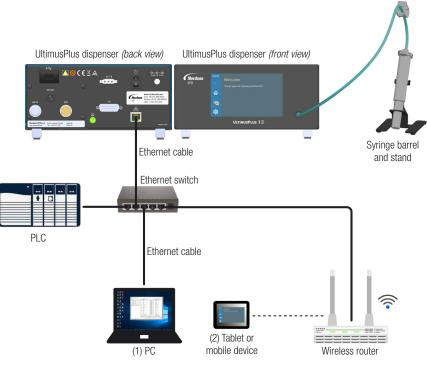
Example setup for UltimusPlus dispenser connectivity: (1) Nordson NX Client Application open on a PC (2) NX web interface open on a tablet or mobile device
