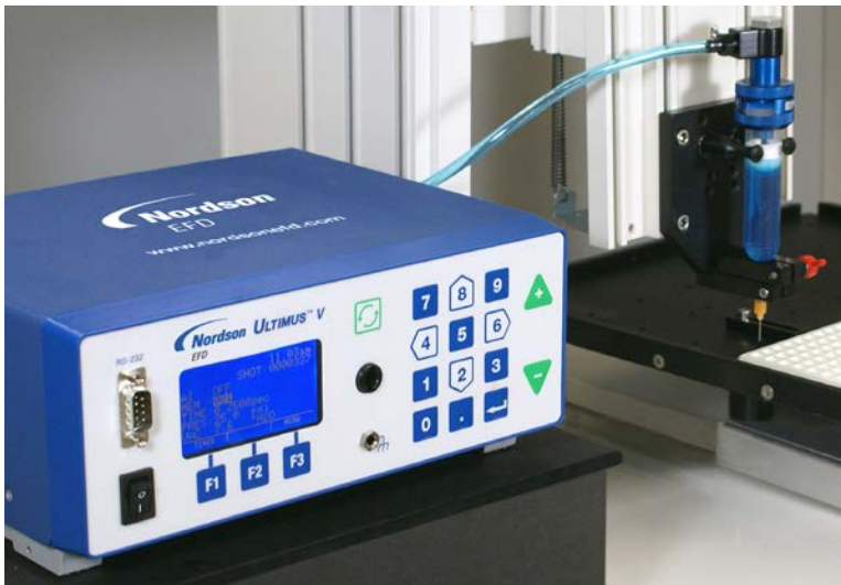
High speed microdot dispensing with Ultimus V and Optimeter.
